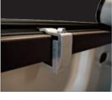
No-drill installation clamps secure frame rail assembly to bed
