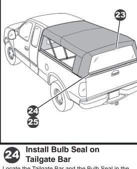
Locate the Tailgate Bar and the Bulb Seal in the parts kit. Slide the channel in the Bulb Seal over the ledge on the Tailgate Bar.
