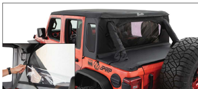
Zippered mesh window for additional air flow.
