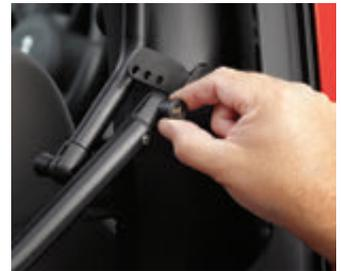
Adjustable bow system helps keep fabric taut and includes Bestop® quick-release bow knuckles
