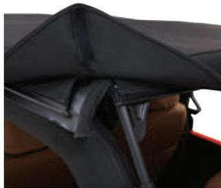
New folding frame design lets the Trektop™ Glide™ fold back behind the rear seat for a total open-air ride or pull forward when you want full coverage
