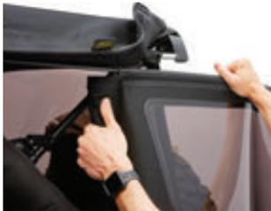
Combination of zippers and zipperless channels makes window install and removal seamless
