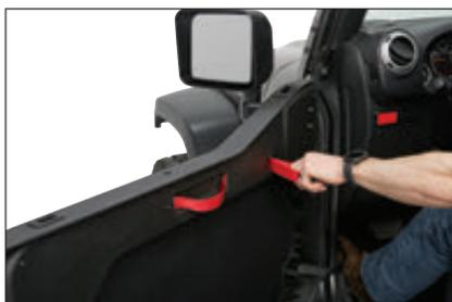
Remote latch release and OEM-quality check strap
