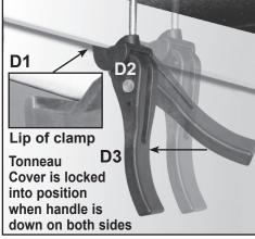
**8b**. To clamp cover down, put lip of clamp hooks under the side metal bed rail and push handle down. (See D1, D2, D3)
