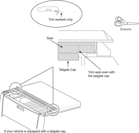
If your vehicle is equipped with a tailgate cap, you will need to trim the seal on the Tonneau Cover Assembly. Mark the seal at each end of the tailgate cap and use the scissors to trim the bottom part of the seal at the mark.
