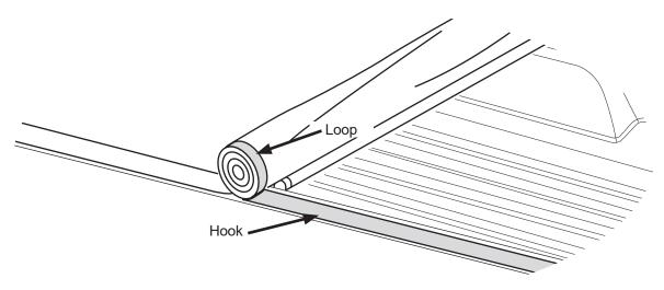
Pull the loop (on the fabric) tight from side to side to the hook (on the rail)
