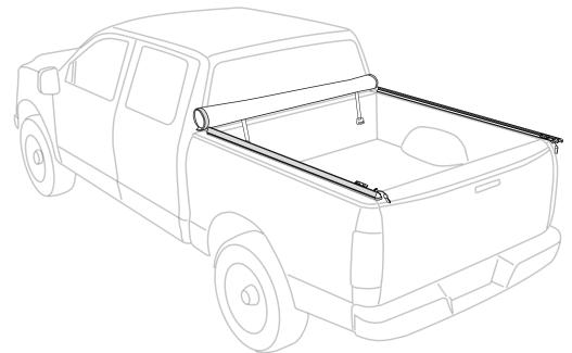
Un-roll the cover and latch the tailgate retainer
