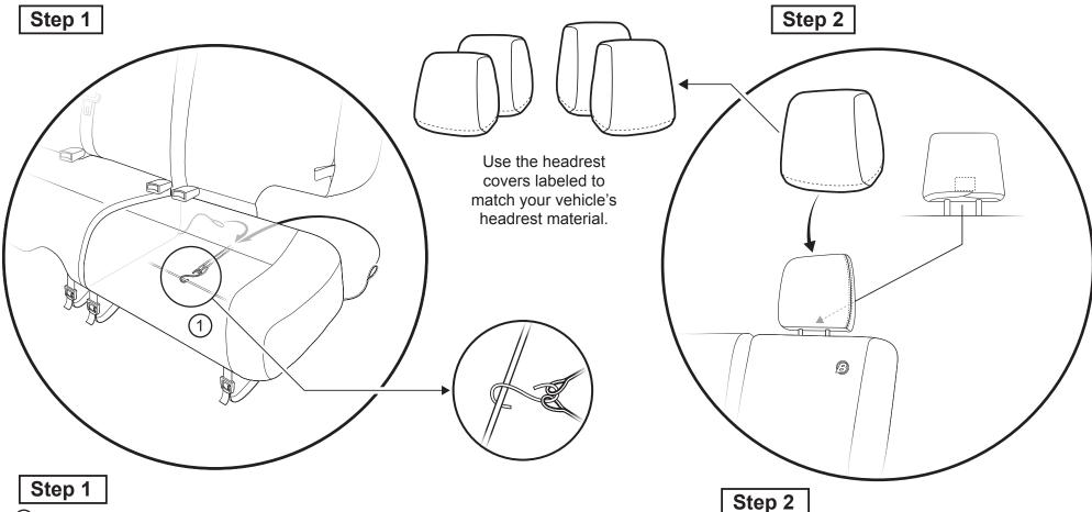
1 Attach the two ends of the elastic cords on the Small seat bottom cover to the closed end of one of the s-hooks.
