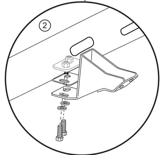
① With help, lift the Side Step onto the vehicle aligning the Center Mounting Bracket and the Rear Mounting Bracket to the studs located on the body mounts. Loosely replace the nuts that were removed in Section 1.
