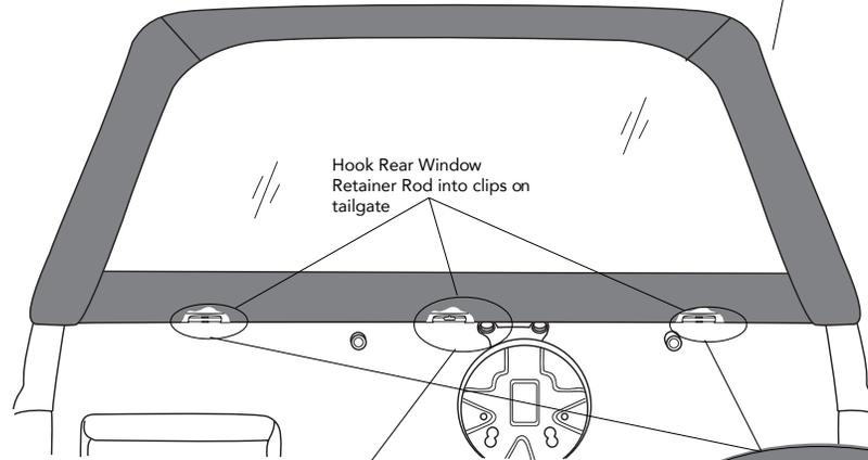
Detail of Rear Window Retainer Rod into center tailgate bracket
