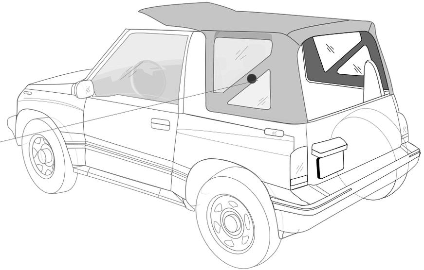
*Note: To open Side Window Retainer, pull out and up on the retainer to release it from the clip mounted to the body.*
