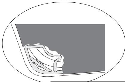
*Note: To close Side Panel Retainer, push the retainer into the clip mounted to the body.*
