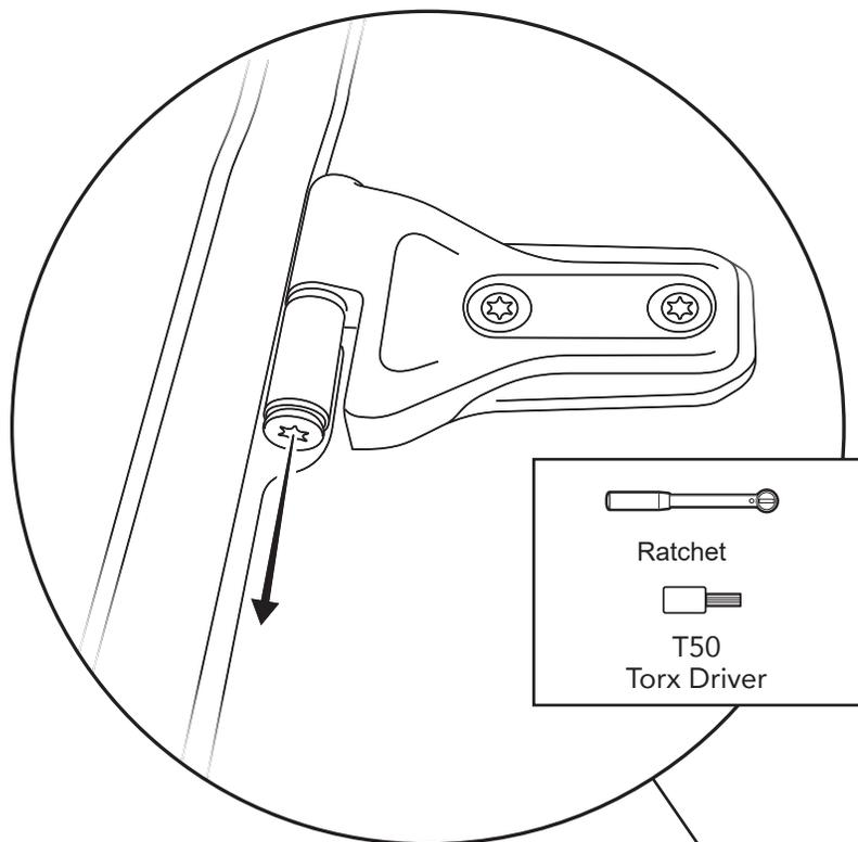
Using a T50 Torx bit, remove the Hinge Screws from the bottom of each door hinge - 2-door or 4-door.
