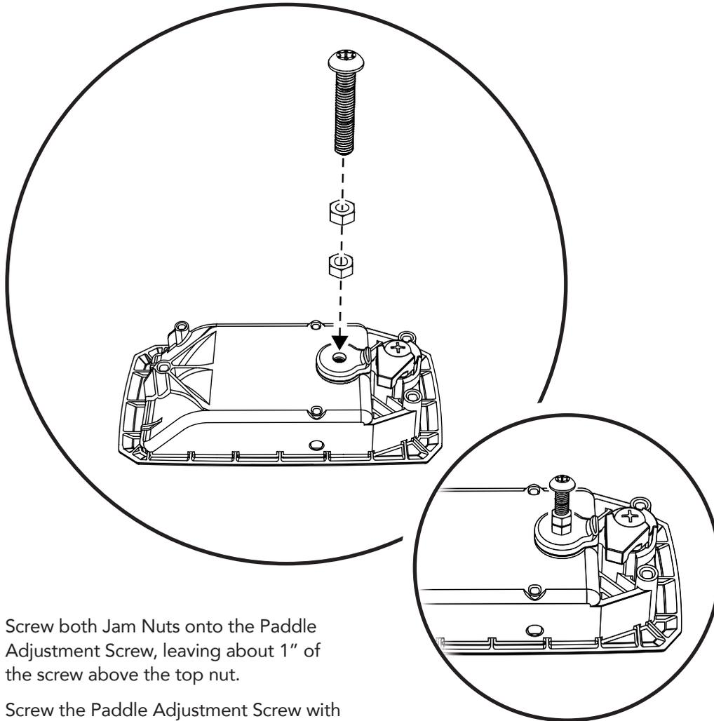
Screw both Jam Nuts onto the Paddle Adjustment Screw, leaving about 1" of the screw above the top nut.
