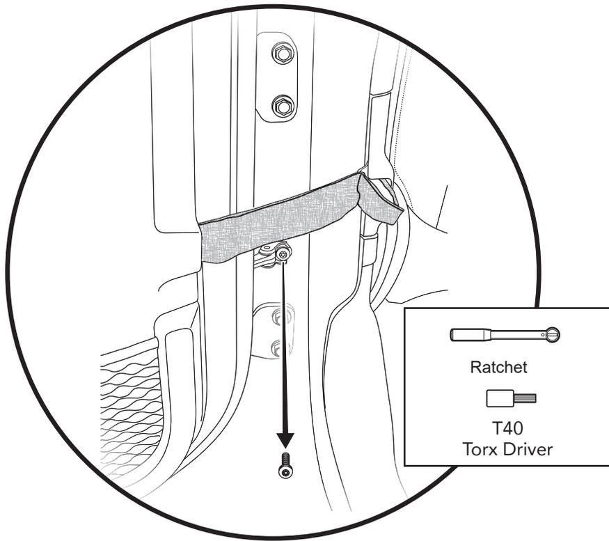
Using a T40 Torx bit, remove the door linkage screw on the inside of the door frame.
