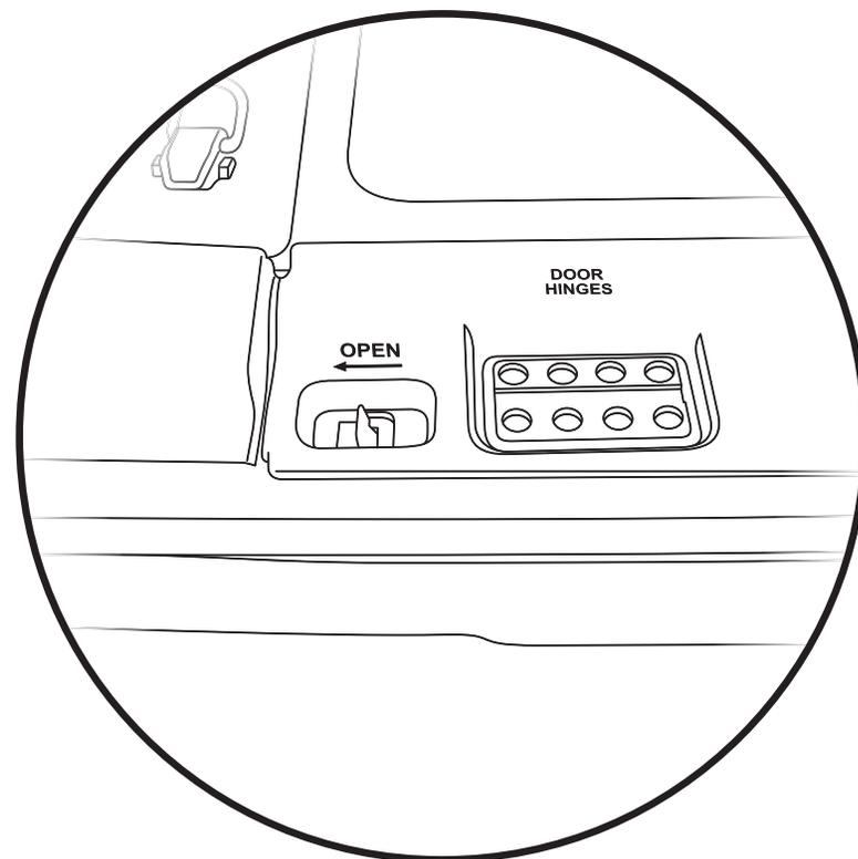
Store the Door Hinge Screws underneath the hinged floor cover at the rear of the Jeep.
