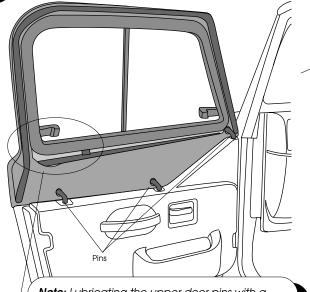
**Note:** Lubricating the upper door pins with a light weight oil will make it easier to install and remove the upper door.
