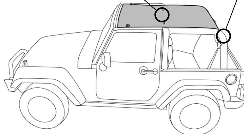
Lay the rear straps around the outboard side of the Sport Bar. Wrap the strap around the bottom of the rear seat belt D ring bolt and up and through the buckle in the Sun Bikini. Pull the straps tight.
