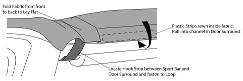
Note: When removing the Bikini, it will be easiest to remove the plastic strips by starting at the front of the plastic and pulling down and out.
