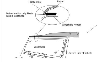
**Note:** For best possible installation, check to make sure that the soft top is perfectly centered on the vehicle.
