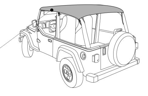
Locate Hook Strip between Sport Bar and Door Side Rail and fasten to Loop
