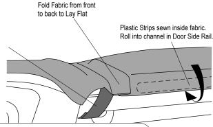
**Note:** When removing the Safari Bikini, it will be easiest to remove the plastic strips by starting at the front of the plastic and pulling down and out.
