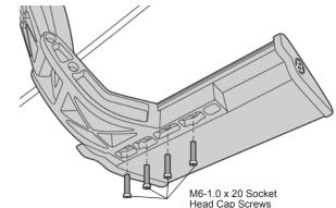
**NOTE:** If step hits the side panel when retracted, proceed to next page to install the 2" spacer. Some models require step to be lower.
