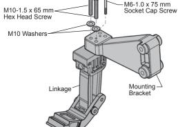
4 Install Linkage Assembly
