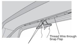
Drill 0.136" Hole and install #8 x 1/2" Self Tapping Screws
