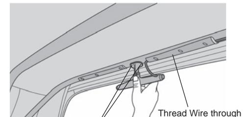
Drill 0.136" Hole and install #8 x 1/2" Self Tapping Screws
