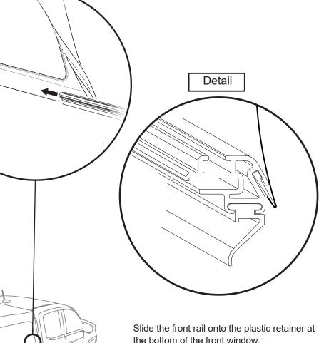
Slide the front rail onto the plastic retainer at the bottom of the front window. The rail should go under the large flap.
