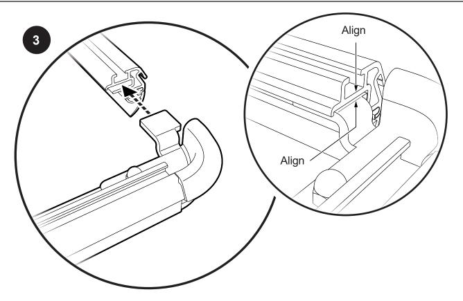
Attach the Front and Rear Rails to the Side Rail Assemblies.
