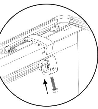
Align the Pre-installed Upper Clamp to the Lower Clamp, using Hex Bolt to tighten the two Clamps together.
