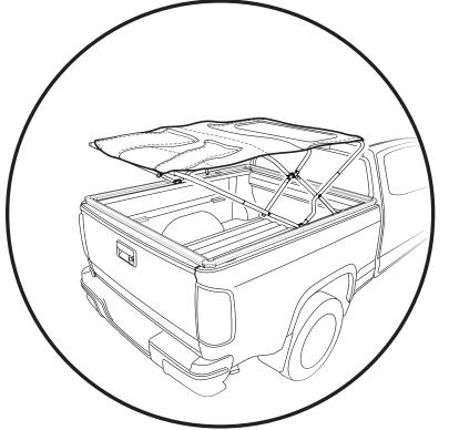
Place the folded Soft Top onto the unfolded Bow Assembly.
