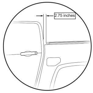
Place the outer edge of both side rail corners 2.75 inches from the back of the vehicle cab.
