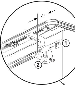
Remove the end cap from the vehicle track system, and slide the Track Block into the track.
