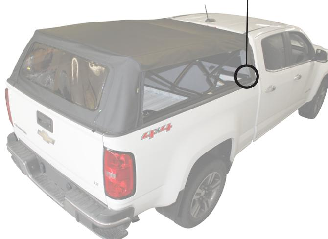
Slide the Front Rail into the sleeve at the bottom of the Front Window, and re-attach it at the front of the Side Rails.
