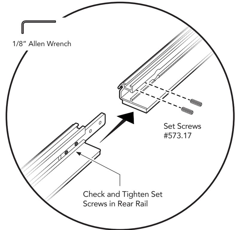
Assemble the Left Front Side Rail and the Left Rear Side Rail.
