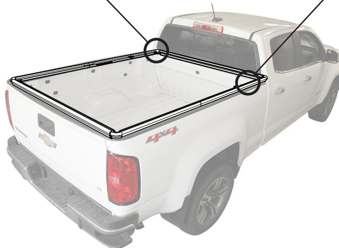
Align the edge of the flanges at the front of each Side Rail Assembly with the forward edge of the recessed line in the top of the plastic bed protector, as shown in the diagram above.
