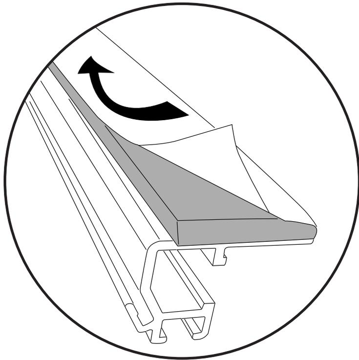
Locate the Foam Tape on the Left and Right Side Rails, and remove the paper backing from the foam tape.
