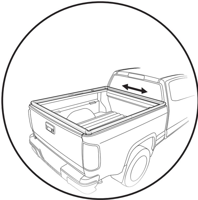
Adjust the Side and Front and Rear Rail assembly right-to-left to center it on the bed width.
