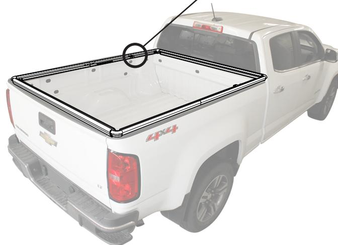
① Attach Clamp Pads to the Upper Clamps on the Front Side Rails, on the rib farthest from the rail.
