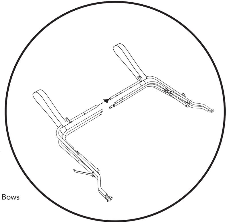
Attach Bow Couplers and to the Passenger Side Bow Stack.
