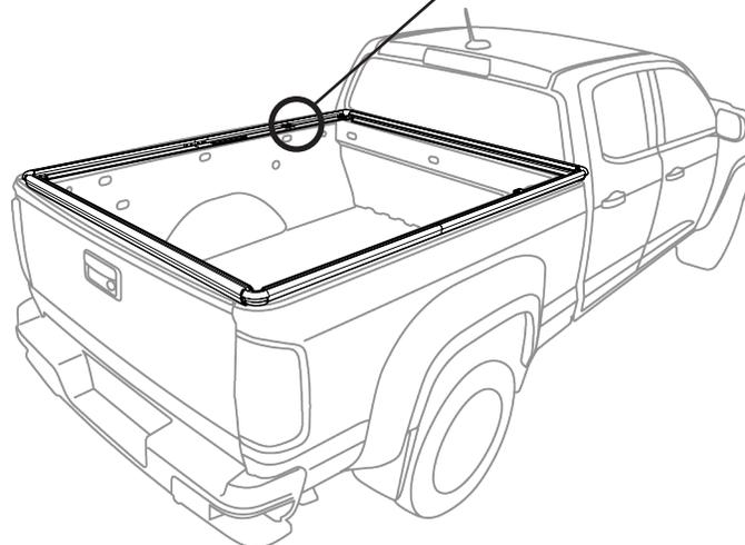
① Attach two (2) Rubber Pads together, and stick them to the Front Rail Clamp, between the rib farthest from the rail, and the next rib.
