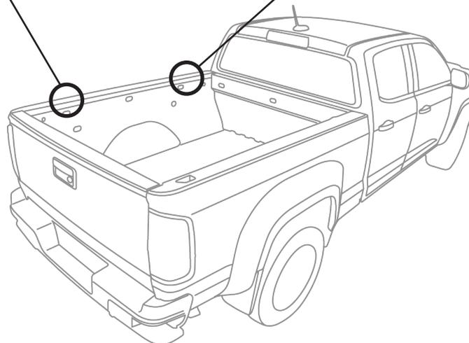
① Attach Lower Clamps to all six (6) pre-assembled Upper Clamps on the Side Rails, using one (1) Hex Head Bolt for each clamp.
