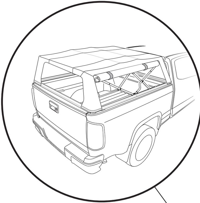
With the Fabric Top up, the Side Curtains can be rolled up and secured with Roll Up Straps.
