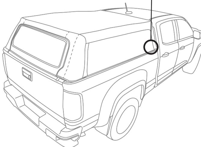
Slide the front rail onto the plastic retainer at the bottom of the front window. The rail should go under the large flap.
