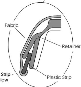
Detail of Plastic Strip - Cross Section View
