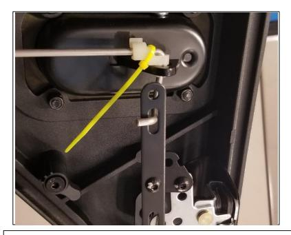
Apply the ziptie **(PN: 605.49)** to each door exactly as shown. Locking feature should be on the lower side of the parts, so it does not interfere with the upper door grommet.
