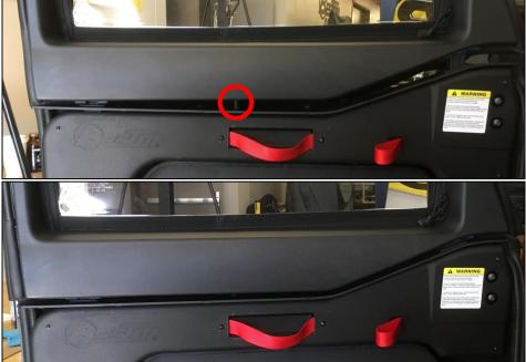
Make sure that the window is fully seated before trying to shut the door.
