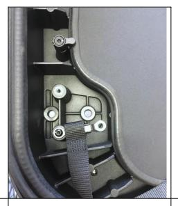
Here you can see the check-strap moved aside, and the bolts holding the hinge have already been removed.
