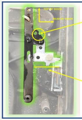
ORIENTATION OF BRACKET- NOTCH FACING REAR OF DOOR AND NOTCH FACING TOP OF DOOR
