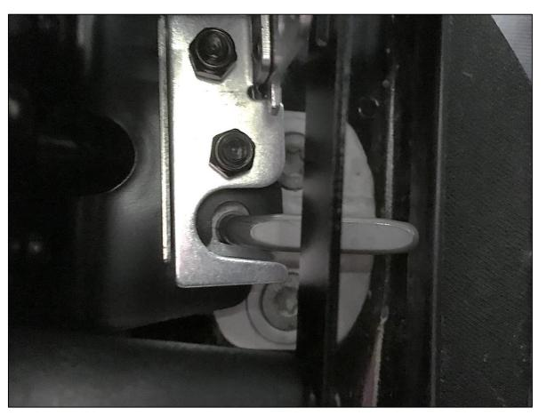
Looking in, you should be able to see the striker hoop centered within the latch, and the latch should be fully closed.
