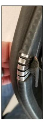
After removing the clips, the knob can be reinstalled with the 4mm hex screw
