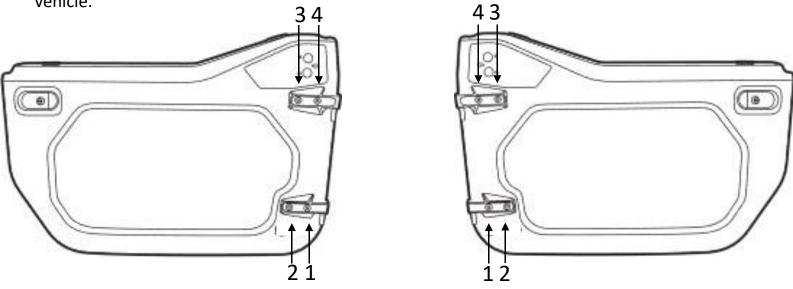
The nuts need to be tightened to **64NM or about 47Ft-lbs**. (This should feel very tight)
