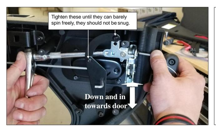
Using a 10mm wrench and a 4mm hex key, tighten the two bolts marked in the diagram while pushing the latch down and towards the door.
