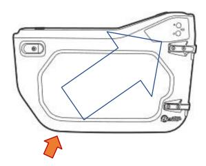
The shim should be placed at the back of the door, away from the hinges, near the rocker panel seams.
