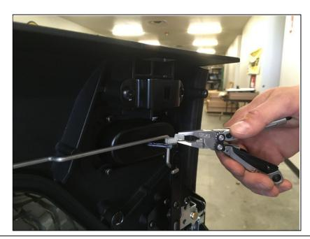
Carefully unclip from the horizontal portion of the rod. The clip should swing open and remain attached on the vertical portion. Using a pair of pliers, squeeze the open end shut and release. Then reconnect the clip to the rod. The goal is to give the clip a tighter grip and ensure it does not vibrate loose or come off on its own.
