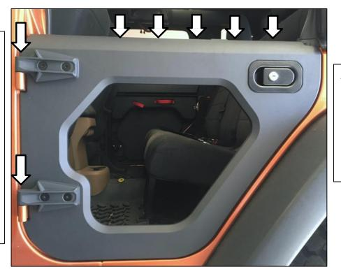
A good way to do this is to reach over the door with your right arm and use your weight to apply the downward force as you tighten the nuts. Use you left hand to hold the hex bolts still and hold the top part of the hinge flush against the lower.
