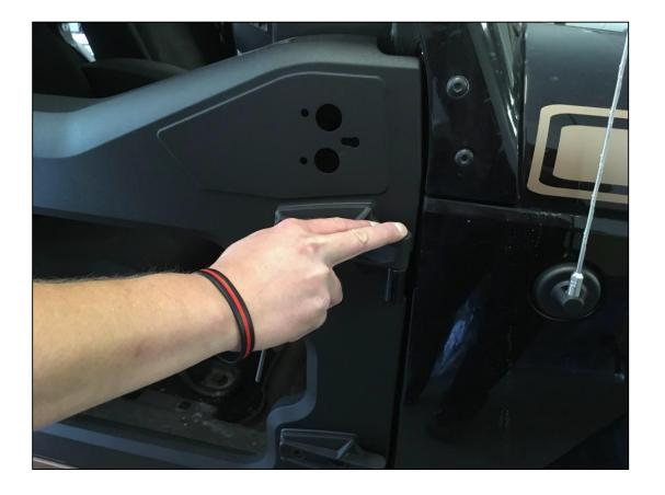
The pressure needs to be applied to the top of the hinge pin, there should be no visible gap between the portion of the hinge attached to the door and the portion attached to the Jeep. This is required to ensure that the hinges support the door when the shim is removed without shifting or sagging.
